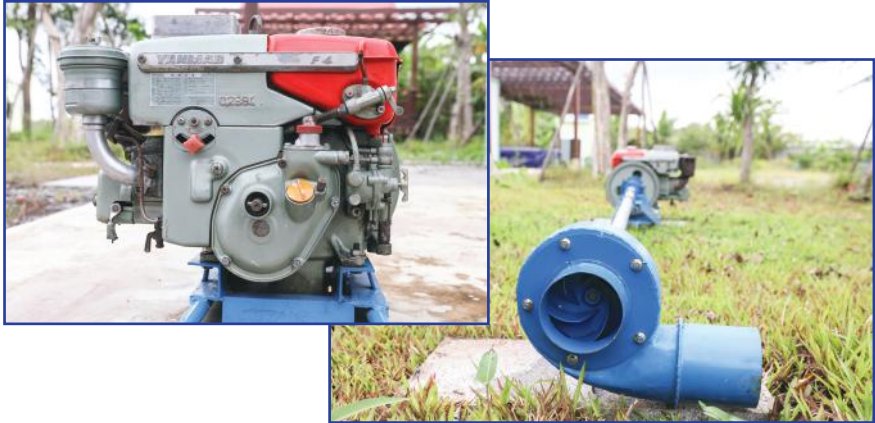
Yanmar (Japan) engine, which was repurposed from a boat engine by removing the propeller from the shaft to be equipped with a centrifugal pump.
