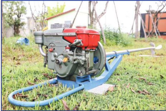
For illustration: Yanmar engine equipped with a propeller as a boat engine
